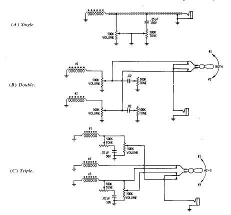
Fig. 2-4. Pickup circuits.
