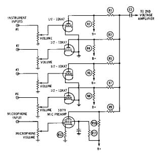
Fig. 2-17. Typical circuit for a 4-channel mixer.
