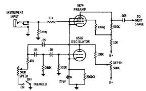
Fig. 2-7. Phase-shift ascillator tremolo circuit.
