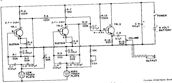
Fig. 2-22. Schematic diagram of an electronic bongo.
