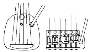
Fig. 2-13. Mechanical vibrato units.
