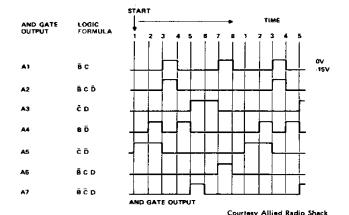
Fig. 2-27. AND gate output waveforms.
