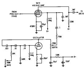
Fig. 2-10. Tremolo signal coupled to screen grid.
