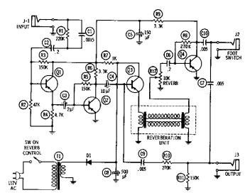
Fig. 2-16. Transistor reverberation unit.
