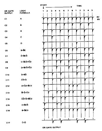
Fig. 2-29. OR gate output waveforms.
