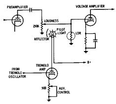
Fig. 2-11. Light dependent resistor (LDR) used to couple tremoto to signal channel.
