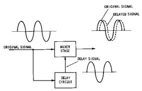
Fig. 2-14. Using signal delay to produce echoes.
