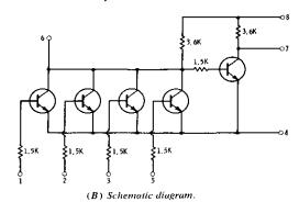
Fig. 2-18. Motorola HEP-581 4-input gate.
