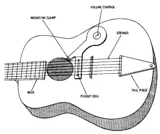
Fig. 2-3. Acoustic guitar with pickupcoil attachment.
