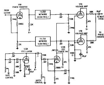
Fig. 2-9. Tremolo appiled as two outof-phase signals.
