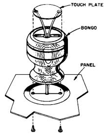
Fig. 2-23. Touch-plate capacitive switch used in the bongo.
