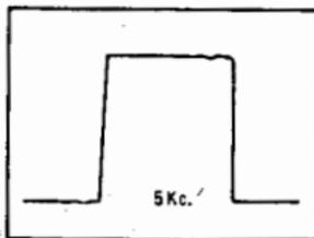
This is a square-wave tracing of the U.L. amplifier at a frequency of 5 Kc. It shows almost complete absence of overshoot and ringing, and illustrates the good over-all frequency response.
