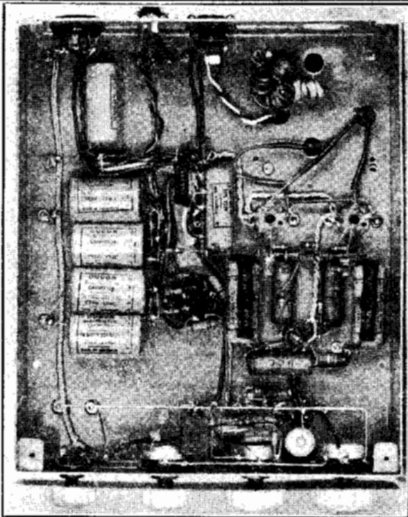
This picture is referred to in the article and shows clearly almost every component. It is the pentode amplifier—the U-L version has only two main filter condensers, shown at the left. Note the corner brackets which help to mount the shield over the front end. Symmetrical layout has been aimed at.
